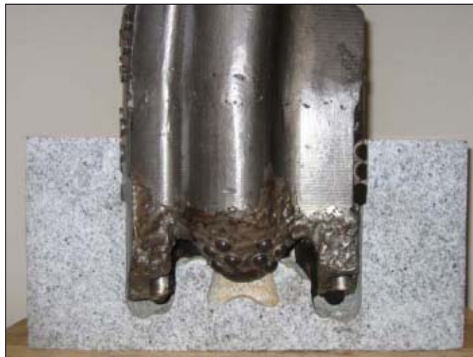
Testing at TerraTek Inc. in July 2005 demonstrates that the PID bit cuts a near-gauge hole (Fig. 3a at left). A cross section of the test block shows the volume excavated by the impact of the steel particles (Fig. 3b at right; photos from Particle Drilling Technologies Inc.).
