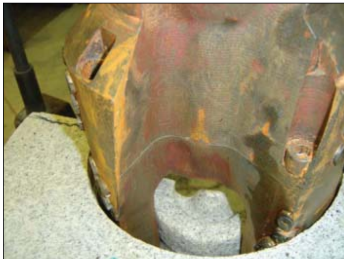
Testing at TerraTek Inc. in July 2005 demonstrates that the PID bit cuts a near-gauge hole (Fig. 3a at left). A cross section of the test block shows the volume excavated by the impact of the steel particles (Fig. 3b at right; photos from Particle Drilling Technologies Inc.).
